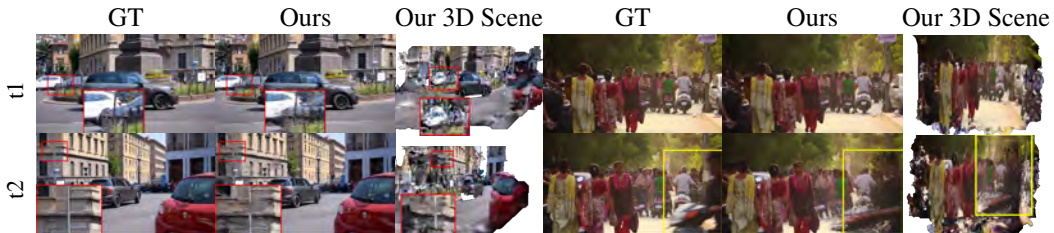
Figure 9: Our method may underperform in two scenarios. (1) Without camera estimation, it has to learn large camera rotations as scene motions, causing distant background blur (left). (2) It fails to track fast-moving transients, as photometric loss is insufficient for motion fitting (right).
