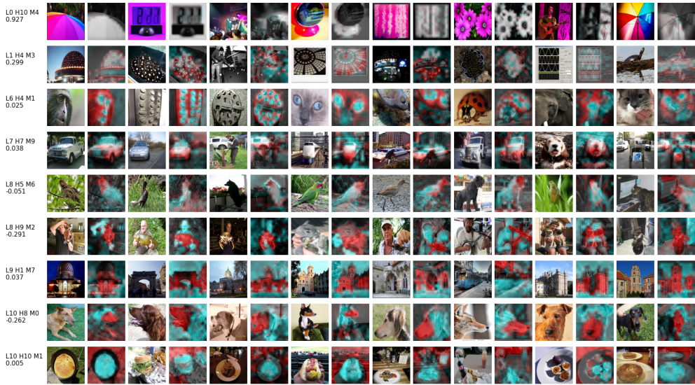
Figure 4: Examples of optimal attention images of singular modes and query and key map in dino-vitb16. Optimal attention images are found from the Imagenet validation set that induce the largest attention score (sorted by the product of the maximum of query map and maximum of key map). The red and cyan channels are the projection values of embedding onto the left and right singular vectors of a singular mode. They correspond to query and key. The white area is where the query map and key map overlap. The name code we assign to singular modes specifies the layer, head, and mode numbers. For example, "L1 H4 M3" means layer 1, head 4, and mode 3. The value below indicates the cosine similarity between the left and right singular vectors.
