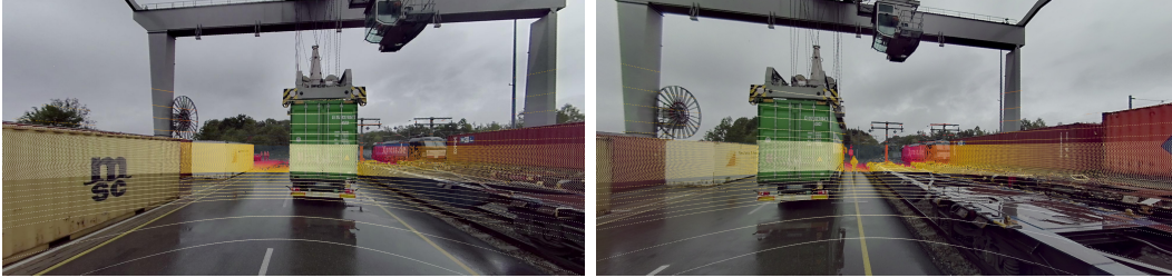
Figure A3: Projection of the left lidar sensor onto the front left camera image (left) and the right lidar sensor on the right front camera image (right). The color of the points indicates the relative distance.
