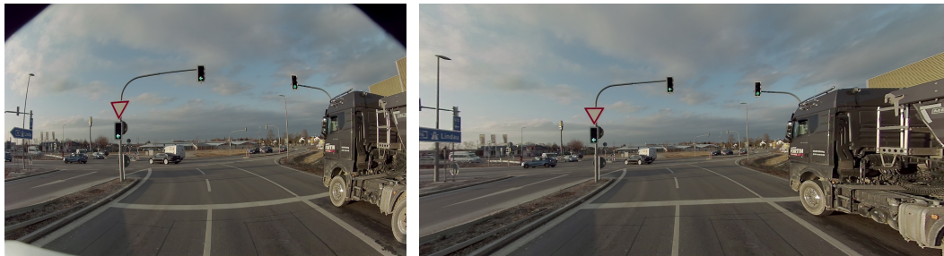
Figure A4: Comparison of the original (left) and the undistorted (right) camera image.
