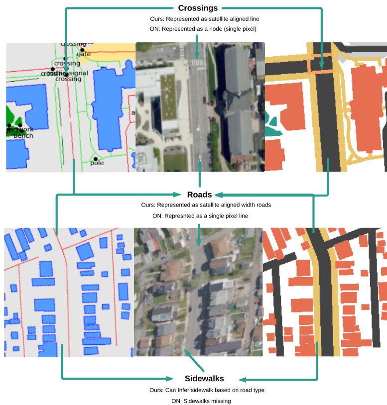
Figure 12: Detailed comparison of BEV rendering/rasterizing pipelines between OrienterNet[33] (left) and Ours (Right). Our road widths are more satellite aligned than OrienterNet’s roads which are single pixel lines. Our crossings are drawn out from sidewalk to sidewalk whereas OrienterNet crossings are single pixel nodes. We are able to infer sidewalks based on road type in accordance with the OSM standards whereas OrienterNet does not.
