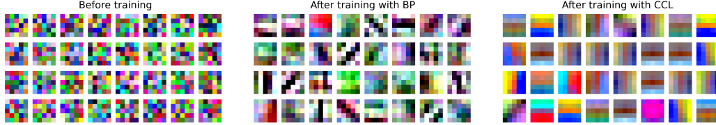
Figure 4: Visualization of the First Layer Convolutional Kernels of the Forward Model Trained with Error Backpropagation (BP) and Counter-Current Learning (CCL). Kernels from models trained with BP have more high-frequency components, as manifested as neighboring white (e.g., weight with high values) and black pixels (e.g., weight with low values). In comparison, those with CCL have more low-frequency components. We posit this might be because the error signal can contain more high-frequency information than the ideal target signal.
