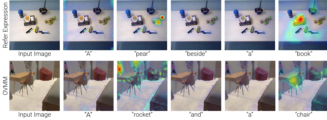
Figure 9: The Stable Diffusion model allows us to extract word-level cross-attention maps for any given text prompt. We visualize these maps in a robotic manipulation environment and observe that they are accurate at localizing objects in a scene. Since these maps are category agnostic, downstream policies should become robust to unseen objects at test time.
