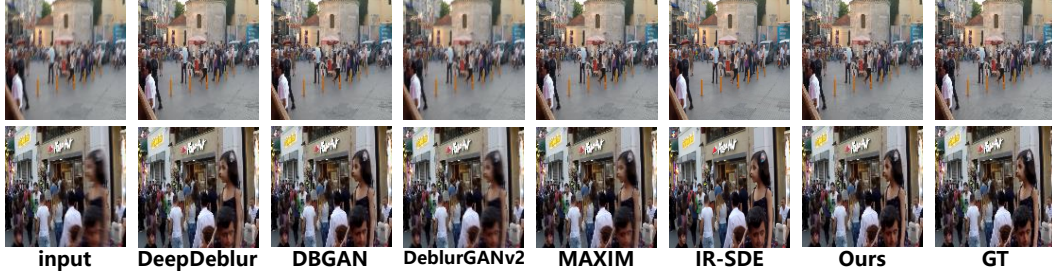
Figure 4: Qualitative comparison results on GoPro dataset. More visual results are available in appendix D.
