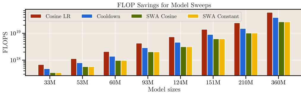
Figure 24: FLOPs savings for all models in scaling experiments across different runs (log scale). The savings amount to a factor of \frac{1}{2} across all models. If more runs across different lengths were to be performed (compared to 3 per model in our experiments), the difference would be even more significant.
