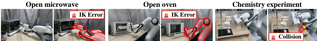
Figure 5: Examples of failure cases.
