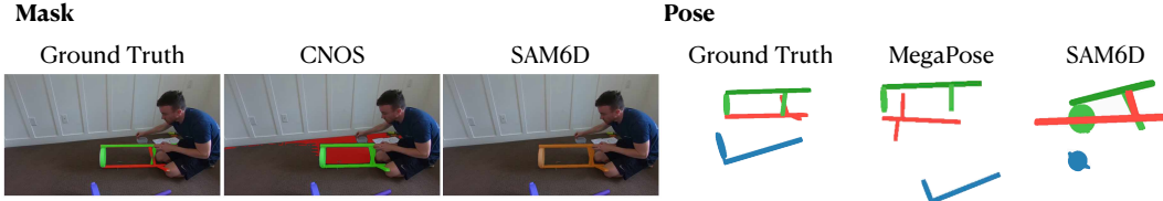
Figure 6: Qualitative Examples. Examples of part-conditioned segmentation (left) and part-conditioned pose estimation (right) on the IKEA Video Manuals dataset. For segmentation, the ground truth masks are shown along with predicted masks from CNOS [37] and SAM-6D [38]. The orange mask shown in the SAM-6D result is caused by the overlap of red and blue masks. For pose estimation, the ground truth 6D pose is shown along with predicted poses from SAM-6D and MegaPose. [39]
