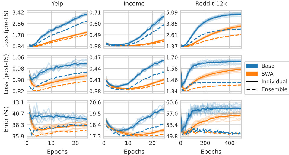
Figure 10: Test curves for 3 real-world noisy datasets. Note that the pre-TS loss is significantly higher than the post-TS loss. Examples of post-hoc reversal between the base curves given by the solid blue lines and the post-hoc curves given by the dashed orange lines (SWA ensemble): (1) optimal epoch is different for base and post-hoc curves for error and post-TS loss on all datasets; (2) for error on Yelp, base curve shows double descent but post-hoc curve does not; (3) for error on Income, base curve overfits catastrophically at approx. epoch 5 but post-hoc curve continues improving till approx. epoch 20; (4) for error on Reddit-12k, base curve does not show double descent but post-hoc curve does.
