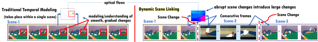
Figure 4: Traditional temporal modeling vs Dynamic scene linking. Notice the abrupt scene change, which causes disruption in visual flow, resulting in large amplitude and widespread optical flow.
