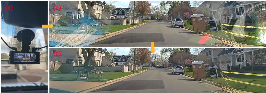
Figure 1: Given a sequence of video captured by a dash cam that may contain obstructions like reflections and occlusions, DC-Gaussian achieves high-fidelity novel view synthesis getting rid of the obstructions. (a) dash cam; (b) original video frame; (c) novel view rendering with obstruction removal.
