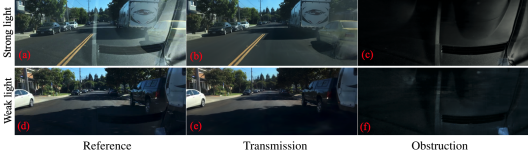
Figure 4: When the intensity of incident light changes, the strength of reflections also changes accordingly (a, d). Our method achieves high-fidelity reflections synthesis (c, f) and reasonable decomposition results (b, e) under varying light. The reflections in (f) are too weak to be seen by the eye, so we brighten it to reveal the details.
