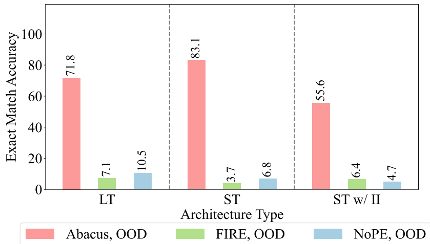
Figure 8: Accuracy of models on the bitwise OR task when trained on data with size up to 20, varying over different positional embeddings and architectures. Abacus Embeddings heavily improve performance on this task.
