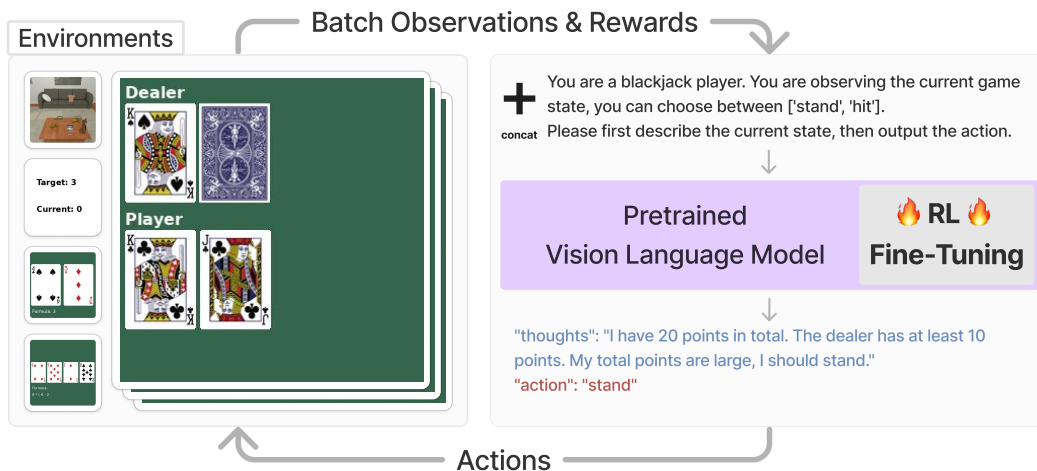
Figure 1: Method overview. We propose a framework for training large Vision-Language Models (VLM) with Reinforcement Learning (RL). At each time step, the VLM takes the current observation and a predesigned prompt as input and outputs an utterance containing a chain of thought reasoning and a text action . The text action is parsed into an executable action to interact with the environment for generating task rewards. Finally, we apply RL with the task reward to fine-tune the entire VLM.
