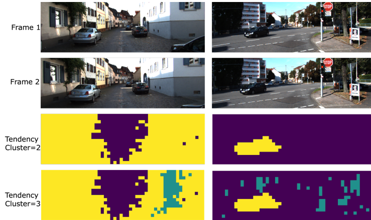
Figure 11: Tendency feature visualization using KITTI dataset
