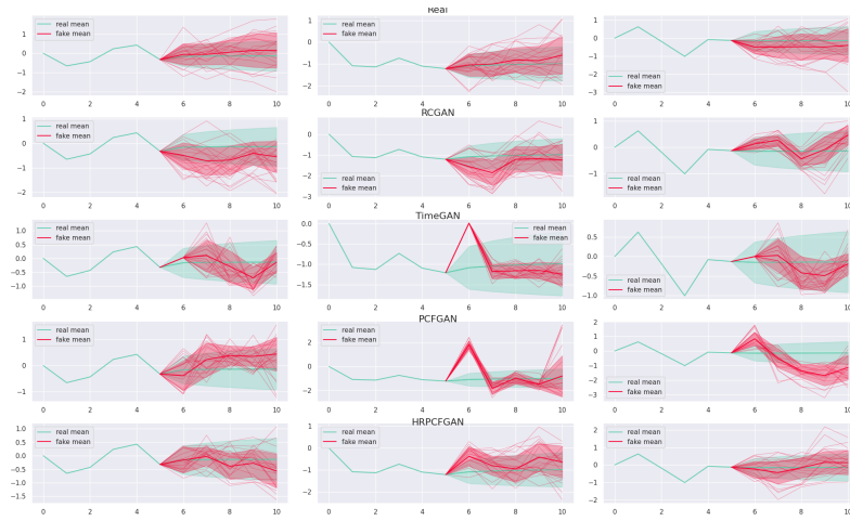
Figure 6: Sample plots from all models on fractional Brownian Motion conditioned on the same past path. The thick red line indicates the conditional mean of future estimated by fake samples, whereas the shaded red area presents the region of \pm std. The thick green line corresponds to the theoretical value for the future expectation and the shaded area shown corresponds to the region of \pm theoretical std.
