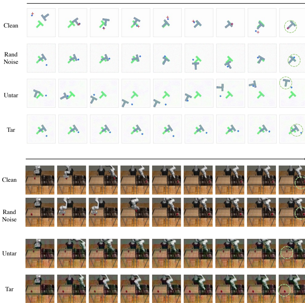
Figure 3: Global Attack (Online) : We visualize the global attacks in Algorithm 1 within both the PushT and Can environments. Specifically, we present action rollouts for four types of observations: clean observations, observations perturbed with random Gaussian noise, and our optimized perturbations (both untargeted and targeted). While the DPs show robustness to random perturbations, they are vulnerable to adversarial samples generated using DP-Attacker.
