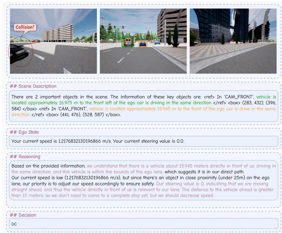
Figure 18: Failure case of collisions caused by other vehicles.
