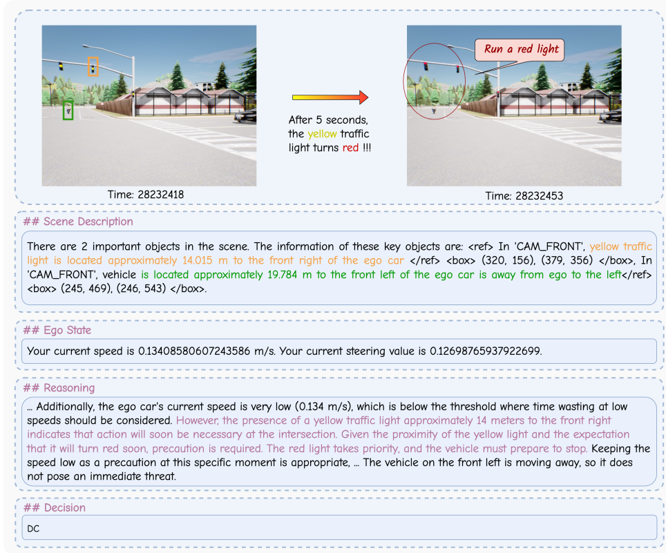
Figure 17: Failure case that running the red light.
