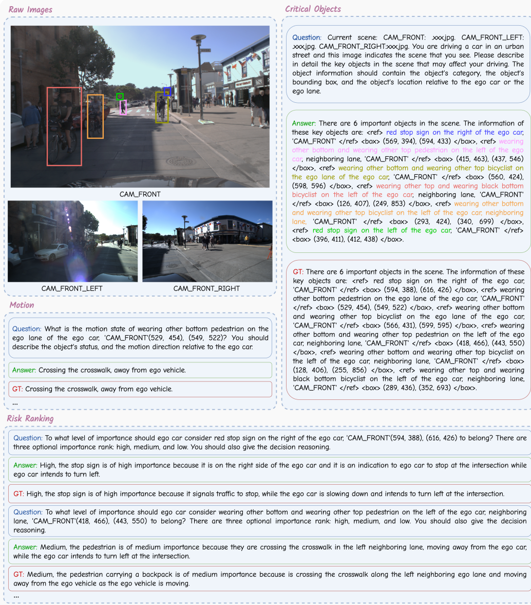
Figure 8: Annotation format and example of scene description generated by VLM on Rank2Tell dataset. It demonstrates the robust performance of our VLM in real-world scenarios
