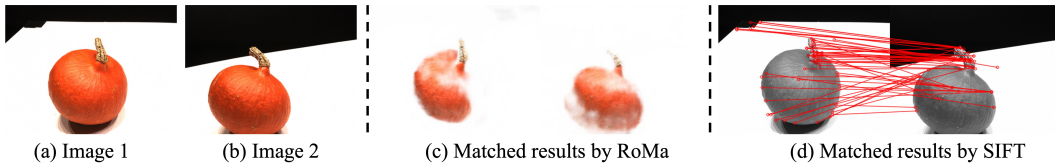
Figure 7: Comparison of the matched results with different feature-matching algorithms. Roma[9] and SIFT[17] implement feature matching between the Image1 and Image2 .
