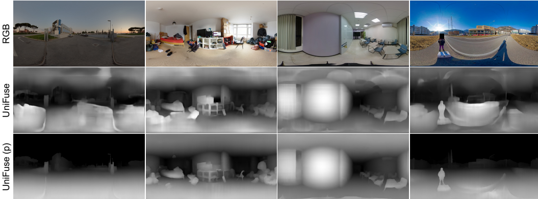
Figure 7: Generalization ability in the wild with depth map visualization. We showcase zero-shot qualitative results using a combination of images we captured and randomly sourced from the internet to assess the model’s generalization ability. For privacy reasons, we have obscured the cameraman in the images.
