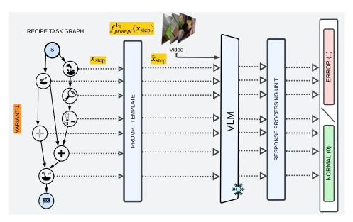
Figure 10: **ZeroShotERV1.** We outline the methodology for the proposed variant  $V_1$  as follows: Initially, we integrated the raw textual descriptions of steps extracted from task graphs into an engineered prompt template to create a single-question prompt specific to each step of the recipe. This prompt, along with the corresponding video, is inputted into a VLM. We analyze the responses generated from the VLM to obtain its predictions corresponding to each step of the recipe.
