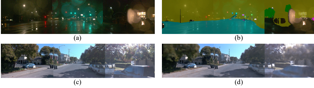
Figure 11: The illustration of the failure cases. It indicates that the image data are influenced by the lighting conditions at night (a), rainy weather conditions (a), and the camera's overexposure condition (c). Then we could not generate accurate detection and segmentation results (b), and reconstruction with lower quality (d).
